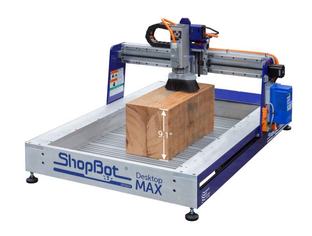
This document will illustrate the differences in maximum bit length, material thickness and cut depth between the standard aluminum t-slot deck option for Desktop and Desktop MAX tools compared to the "Lower Deck" option where the t-slot decking is mounted to the underside of the tool frame. The thickness of the material you're able to cut with each option will depend on the type of cut you're trying to achieve and the style of bit that you've chosen for the cut.
