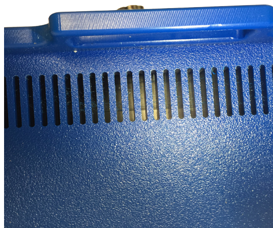
Light shining into vent slots, revealing metallic motor casing.
