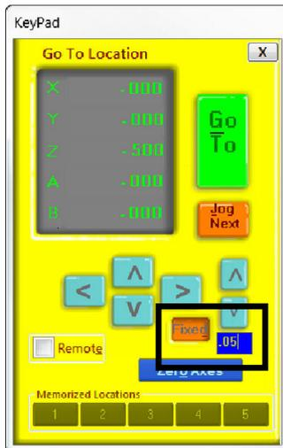
Click on the yellow button in the position window or push the “K” key to pull up the keypad window for positioning and setup of the tool head. Use the keyboard direction arrows or the blue buttons for coarse movements.
