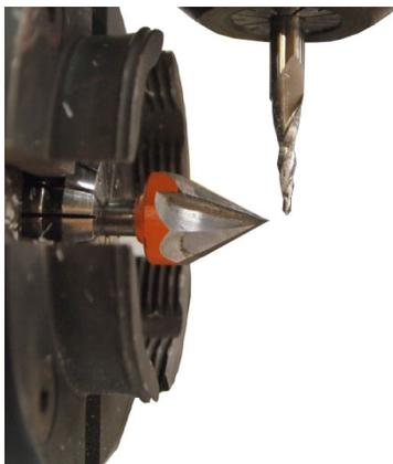
Chuck another fine bit into the spindle. Sharp ended bits allow precise identification of position relative to one another. Use the keypad to move the spindle bit about 1/8” in front of the center bit.
