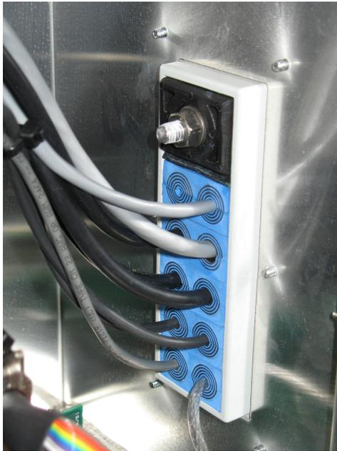
Open the Roxtec cord fixture on the side of your control box. Depending on the age and model of your Shopbot, the fixture is closed either with a bolt on the inside of the box (shown in the photo), or a plastic clamp.
