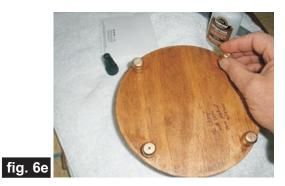
Apply glue into the holes of the base and glue the top assembly onto the base. The taper of each dowel should allow you to easily guide each dowel into the holes. Make sure all the dowels are fully seated before setting aside to dry. (fig. 6f, 6g)
