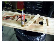
Since this project will spend its duration outdoors, a construction adhesive is used to glue the parts together.
