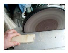
Sanding off the tabs with a disc sander speed up the process of finishing this project.
