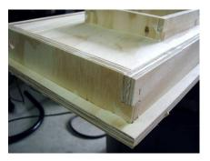
The corners should lap and adding another pin nailer shot into these corners ill add to the strength.
