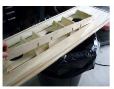
Add the two longer inside pieces and make sure they are pushed down into the grooves.
