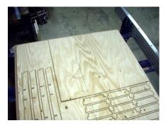
Included in the tool path is a cut off of the scrap piece of material. This allows this piece to be cut aside for future projects.
