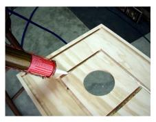
Start by laying a line of adhesive on all of the inside grooves.
