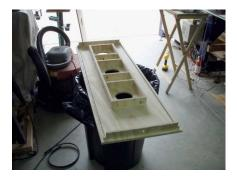
Following the same order of operations add the other pieces by applying adhesive to all of the grooves and then installing the shorter pieces to the ends.
