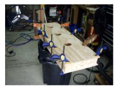
Flip the pieces onto each other and apply clamps. The two halves will now glue up and match each other perfectly.
