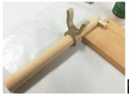
Glue the Hook so the ring meets the mark. Wipe away excess glue with a damp rag. The Hook is positioned at a 90-degree angle from the tenon of part #6.
