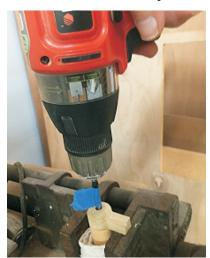
Drill hole into dowel end using existing hole in part #6 as a quide
