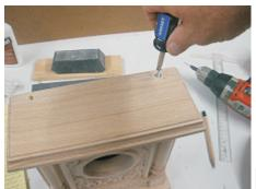
Drive #6 x 1 " wood screws through the holes and into the back panel edges. (fig. 4j)
