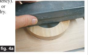
Glue the arch parts together. Clamp until dry. Sand to blend the seams after the assembly is dry. I used a 1" belt sander to make the job go faster. (fig. 4b)
