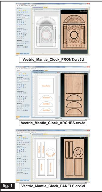
Carefully review all the toolpaths and make any necessary changes to suit your particular bits and machine. The toolpaths are currently set with ordering and feeds, speeds and pass depths that were used in creating the original sample. Please don't use them directly until you review them for your own setup. It is VERY IMPORTANT to recalculate all toolpaths after making any edits/changes. Preview all toolpaths again to visually verify the project outcome on-screen before running the files.
