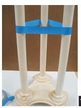
Wrap a strip of painter's tape around the posts, lining up the top edge of the tape with the pencil marks.
