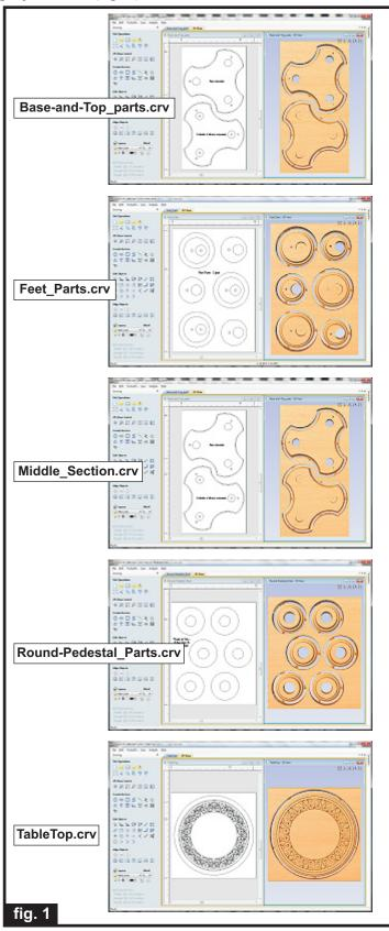
Carefully review all the toolpaths and make any necessary changes (feed/speed, RPM settings, etc.) to suit your particular bits and machine.
