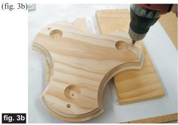
Flip the part over and drill countersinks into the flat underside at the three **inner** pilot hole locations. (fig. 3c)
