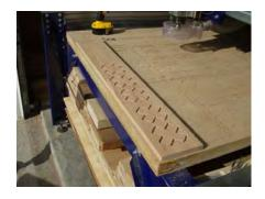
A scrap piece of red oak is used for the X's. Simply locate safe locations for the hold down screws and install one in every corner.
