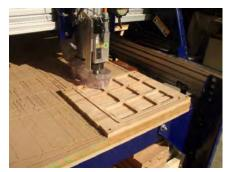
Secure the game board piece to the table surface, for this example screws are put in each corner at a safe distance from the cutting area.
