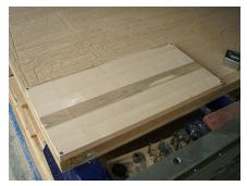
Included with the cut file is a hold down toolpath that shows where it is safe to put screws. Run this file separately from the cut file so you can screw down the work piece, or if you have a different size board or different type of hold down disregard the file. Not all 50 states have hold down files provided.
