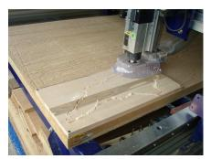
As the file starts cutting the profile of the parts make sure the cut is going all the way through the work piece and into the table surface. If you need to adjust any part of the file make sure you do not remove the hold down or you will loose position.
