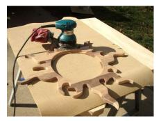
Sand all the edges and faces to ensure the grain is smooth. A random orbital sander works great because one does not have to follow the direction of the grain while sanding.
