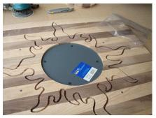
Before unscrewing the part from the table make sure the mirror drops into place. If this does not fit, simply go back to the file and increase the size of the cutout. If hold-down had been removed, one would not be able to line this back up perfectly.
