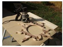
The entire outside of the project is routed with a 1/4" roundover bit. The only edge that is not rounded over is the rabbit on the backside that the mirror drops into.
