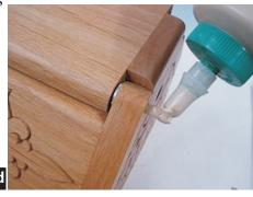
Dry fit the swinging handle using the <sup>5</sup>/8 "dia. and 1 "dia. dowels. Test swing action, then apply wood glue inside the <u>handle</u> round pocket recesses and install the handle components to the box. *No glue* goes into the pockets on the box itself...this is so the dowel/handle assembly will be able to swing up/down freely. (fig. 5e)
