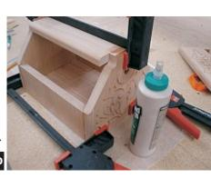
It's a little easier to apply the finish to the inside of the box *before* gluing the top in place. If you choose this method, after the glue dries, remove the clamps and top panel 'spacer', then apply your finish to the box. After the finish is dry, center the top panel between the ends and glue and clamp in place until the glue cures.
