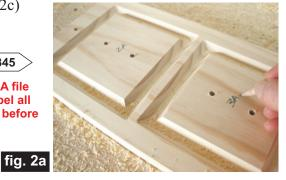
After machining and labeling the <u>SIDE A</u> file, flip the board over <u>across the (shortest) width</u>. Insert two alignment dowel pins into the holes in the spoilboard and replace the board onto the pins with the plain side up. Re-apply a secure holddown method.
