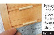
Epoxy two 0.25 "x 1.5" long dowels into the slider grooves of the main base. Position them 1.1875" from the seam of the front strip. (fig. 7i)
