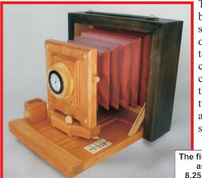
This project makes broad use of the Vectric software's precision drawing tools and toolpath features to create the various camera parts. Four of the bellows parts require two-sided machining to achieve the accordianstyle appearance.
