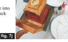
Epoxy the pointer to the underside of the faceplate base (photo does not show this - I forgot until later). Now, epoxy the faceplate base onto the slider dowels and feet of faceplate. Position the faceplate base about 0.125"
