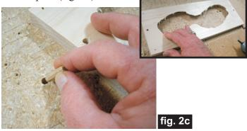
When I ran the next two pairs of files (2a-2b and 3a-3b) the spoilboard holes were already present, so I reduced the depth of the drill toolpaths to just go through the material and used the existing spoilboard holes. Of course, I maintained the same X,Y zero location on the machine bed throughout the complete project run. Inserting a couple dowels into the holes in the spoilboard and into the material holes, yields perfect alignment between the back and front of the material.
