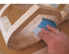
After the assembly is dry, sand the inside with coarse sandpaper to blend the sections. (fig. 4e) fig. 4e
