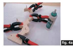
Glue the attachment panel together (the plain side glues to the underside of the piece). (fig. 4b)
