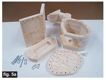
You can insert all the dowel buttons at this time, **or** wait until after the main finish is applied. I opted to brush on the finish, **then** insert the dowel plugs after that. I then "dabbed" the appropriate paint color on the dowel plugs to match.
