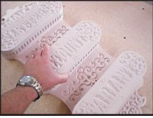
Test-fit the mail holders onto the Main Panel. (fig. 4c)
