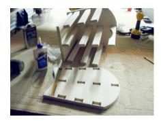
Apply glue to the second end piece and rotate the first assembly onto this. Be careful placing each piece into the respective pocket and use the rubber mallet to lightly tap into place.
