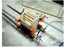
Clamp the assembly for a couple hours so the glue has a chance to setup.
