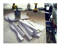
Rub all of the pieces with Minwax Wipe-On Polyurethane. It is easiest at this point in assembly to get an equal coat on all of the pieces.
