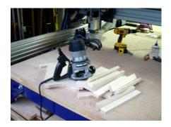
All of the edges except for the bottom of the magazine rack should get a 1/4" round over bit.
