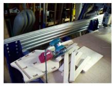
Sand all of the faces and edges to ensure there are no sharp edges or potential slivers sticking out.
