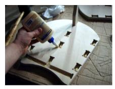
Squeeze some glue into all of the pockets on one of the end pieces. Push the glue around with your finger or a small brush.
