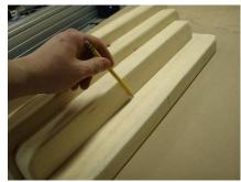
Flush the back pieces with the back edge of the shelf. A scribed line will help show where to place the glue.
