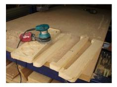
A random orbital sander should be used on all of the surfaces and hand sand paper to knock down the sharp corners. One can also add routed edges if desired.
