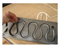
Start with one end and fish the rope through the channel. Make sure it isn't twisted up to much or the rope will have a tendency to pop out of the grooves.
