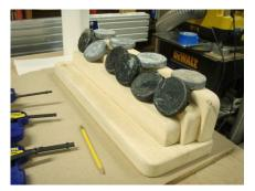
Clamps or weights can be used to attach the back pieces to the bottom of the top piece. Make sure everything is centered and flushed before the glue sets up.
