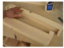
There are no fasteners used for assembling this project, so a proper glue joint is necessary to hold the pieces together. Spread glue evenly on both surfaces.
