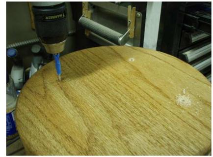
Put some tape on a pilot bit to make sure that when predrilling one does not accidentally drill all of the way through the wood.
