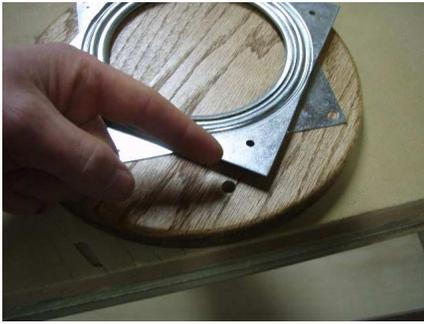
This file comes with 4 holes in the bottom piece that are spaces specifically for the lazy susan hardware used in this picture. The lazy susan purchased by you could have different hole layouts and the file could use some adjusting.
