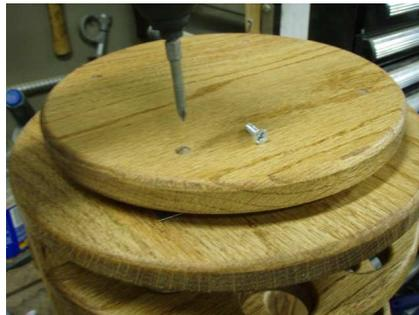
Use the pre drilled holes in the bottom piece to predrill and screw into the rest of the project. Center this by eye. Make sure short screws are used so they don't stick through the other side of the project.
