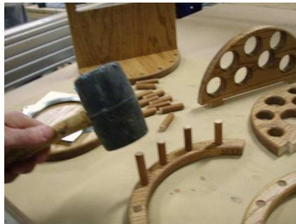
With a rubber mallet tap the dowels into the half moon pieces. Also confirm the dowel that is being used fits into the holes before doing this. Different manufactures of dowels can be off on the diameter slightly.
