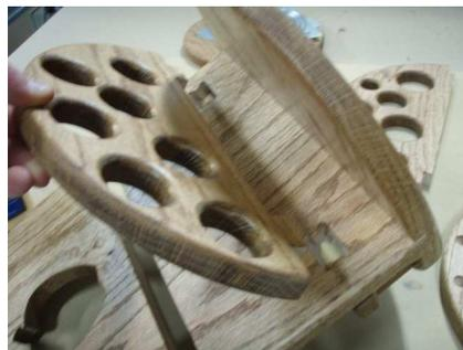
Insert glue into the pockets. Push the shelf into these pockets and allow to dry.
