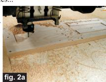
After machining and labeling the <u>first</u> file parts, flip the board over <u>across the (shortest) width</u>.
