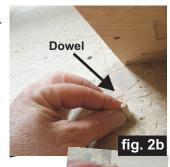
Push board onto the dowel pins for perfect alignment between side 1 and side 2
