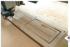
After flipping the material width-wise, run the side 2 file and label the parts after machining
