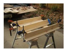
Keep this upside down and clamped until the glue has set. Glue has a tendancy to drip out of the dog bones, doing this will prevent this from happening
