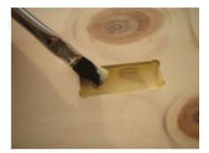
Apply a good amount of glue inside each mortise and rub around with a brush. This gets glue on all of the sides and strengthens the joint.
