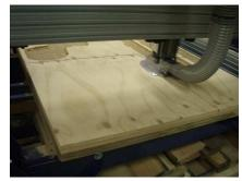
There is an extra toolpath in this file that cuts out a 30" square. This does not have to be done, it is simply put in the file to cut this piece out so it can be used for another project.
