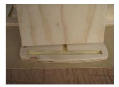
Once the three pieces are attached to the first end piece, let the glue setup before flipping over to the other side or the glue will drip like noted before.
