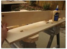
The first assembly step is to assemble the supports to the undersides of the seats and table top.
