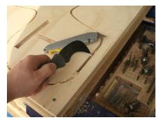
Tabs are use to hold all the pieces to the scrap wood attached to them. Use a utility knife to score these edges. A carpet knife works well to score the tabs before lifting the pieces up. Never try to push a piece out without cutting the tab, it will tear the grain on your project. Sand remaining tab flat.
