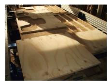
Again, to avoid a 30" x 30" piece from going to scrap, a extra toolpath was added to cut this square out.
