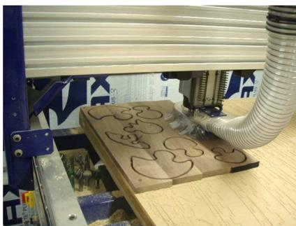
As the file starts cutting the profile of the parts make sure the cut is going all the way through the work piece and into the table surface. If you need to adjust any part of the file make sure you do not remove the hold down or you will loose position.
