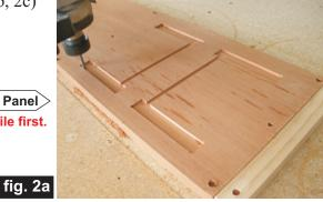
Machine the INSIDE panel file first. After machining that side, flip the board over <u>across the (shortest) width</u>. Insert the two alignment dowel pins into the holes in the spoilboard and replace the board onto the pins with the plain side up and re-apply your hold-down method.
