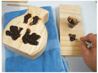
fig. 5i Apply the "stone" into the inlay areas you prefer, as well as a small amount to a scrap board.
