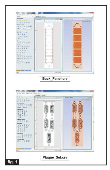
Carefully review all the toolpaths and make any necessary changes to suit your particular bits and machine. The toolpaths are currently set with feeds, speeds and pass depths that were used in creating the original sample. Please don't use them directly until you review them for your own setup.
