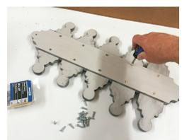
Secure the plaques to the back panel with wood screws (or glue them in place)
