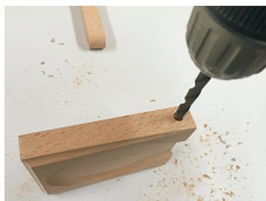
Enlarge the panel holes using a 17/64" bit. This allows the 0.25" dowels to rotate freely within them.
