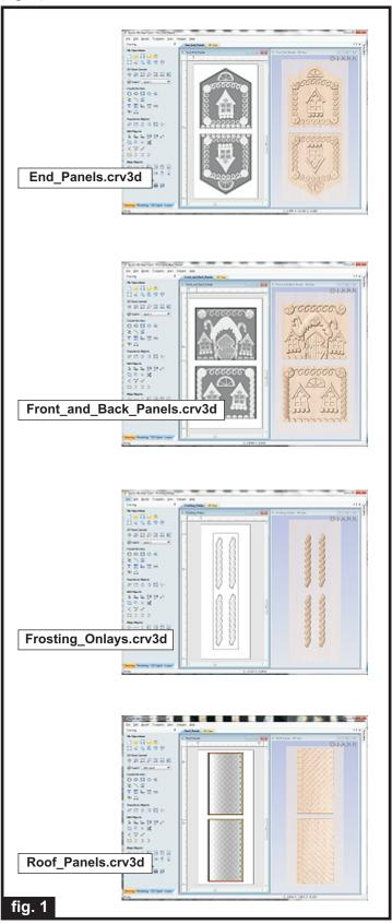
Carefully review all the toolpaths and make any necessary changes (feed/speed, RPM settings, etc.) to suit your particular bits and machine. The toolpaths are currently set with feeds, speeds, pass depths and so on, that were used in creating the original sample. Please don't use them directly until you review them for your own setup. It is very important to recalculate all toolpaths after making any edits/changes.
