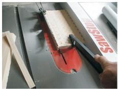
Tape the box together and place atop a board (.5-inch or .75-inch thickness - your choice). Trace along the the inside. Cut this piece to create the bottom of the box. It will be very close to 6 " x 7.25 "(fig. 3e, 3f)
