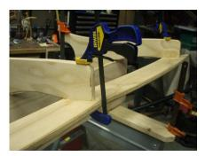
Make sure clamps are used to hold the pieces together until the glue has setup.
