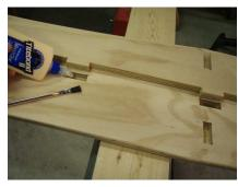
Start by partially filling ALL of the seat mortises with glue. Use a small brush to push the glue onto all of the inner sides. This will make for a much stronger glue joint.
