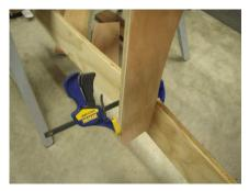
For alignment purposes the backrest is dry clamped into place with no glue. This will help hold the project square while the glue sets up from the previous assembly.
