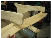
Position the bench so that the glue will not run out of the backrest during the glue drying time.
