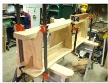
Once the stringer is in place and the three leg pieces clamp this assembly and let the glue dry for the manufactures recommended time. Titebond II is the preferred glue used here. Leave upside down until the glue has dried, or it will run out of the dog bones.
