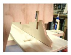
There are three leg pieces. Make sure they fit through the bottom stringer and push down into the seat mortises. Assembling this project upside down is key to a smooth assembly.
