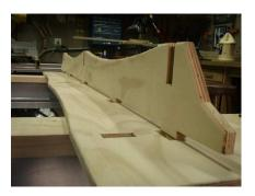
Insert the bottom stringer first. It can go either way, all of the tenons are centered to the seat. Push this down in place before moving to the next step.
