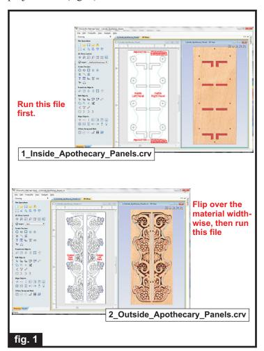
Dimensions for the slots and dowel holes are made slightly oversize to aid in shelf and dowel insertion during glue-up. Be sure to measure your own material to make certain the files' dimensions are suitable for the material you have on hand. It is not at all uncommon for wood thicknesses and dowel diameters to vary by small amounts. Modify the slot and dowel hole dimensions, if necessary. (Recalculate the toolpaths if any changes are made!)
