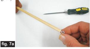
Mark and pierce a pilot hole .75 "from the tip end of the pendulum support arm (on the underside and centered in the middle section). Bend open a small screw eye slightly to form a hook. Screw in the screw eye "hook".
