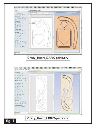
Carefully review all the toolpaths and make any necessary changes to suit your particular bits and machine. The toolpaths are currently set with feeds, speeds and pass depths that were used in creating the original sample. Please don't use them directly until you review them for your own setup.
