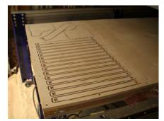
Included with the cut file is a hold down toolpath that shows where it is safe to put screws. Run this file separately from the cut file so you can screw down the work piece, or if you have a different size board or different type of hold down disregard the file.
