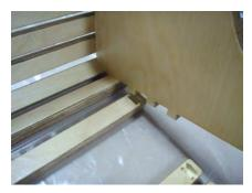
If parts are snug going together, tap with a rubber mallet into place. Make sure a good amount of glue is in the pocket.
