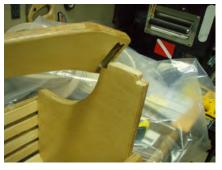
The last step is to glue on the handle. Fill the pockets with glue, tap into place, flip basket upside down and let it sit for 30 minutes.
