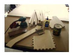
Once the pieces are removed power sand the faces and hand sand any sharp corners. Adding a round over routed edge adds to the eye appeal of this project.
