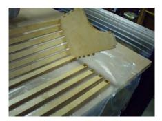
Let the bottom glue rest for about 30 minutes. Then assemble one side and let that sit for another 30 minutes. Repeat this for the other side. Letting the glue rest during this time helps ensure that it will not drip out of the joint.
