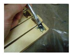
Use a good amount of glue in each pocket. Take a small brush or your finger and cover all of the surfaces in this joint. It is better to have a little extra glue that squeezes out then not enough and the basket falls apart. Squeezed out glue can be easily wiped off.
