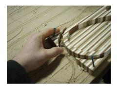
Pay attention to the material thick that you end up using. If it is thicken than the material in the file it would be recommended to beef up the tab sizes. You want them to not break off, but easily cut off with a knife.
