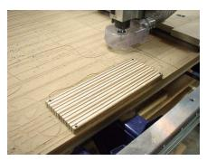
Included with the cut file is a hold down toolpath that shows where it is safe to put screws. Run this file separately from the cut file so you can screw down the work piece, or if you have a different size board or different type of hold down disregard the file.
