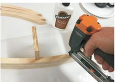
You can use drops of CA glue or pin nailer to tack parts after alignment
