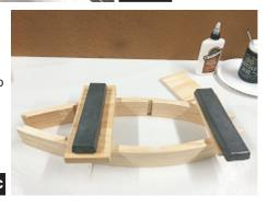
After the glue is dry, final sand the concave and convex surfaces of both hull halves. (fig. 4d)
