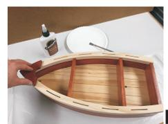
Glue the shelves, trim and tip to the hull assembly. (fig. 6c)
