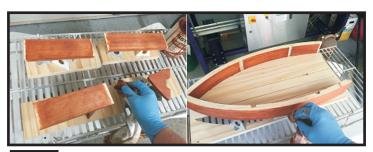
fig. 6a Stain shelves, tip and outer hull (including backside)
