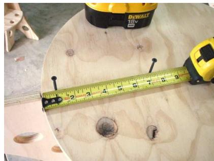
Put a crew in as shown above into the line you traced. Put one in at the 1" and 7" mark. 1 5/8" screws work great for this. Repeat on all four lines.
