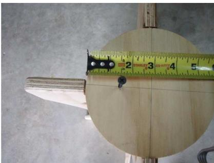
Create a layout line for screws like you did earlier with the table. Approximately 1" in from every edge put a 1 5/8" screw down into the legs.
