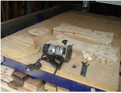
After the tabs are removed and the edges are sanded it is not necessary but adds a lot of eye appeal to route all of the edges with a 1/4" round over bit.
