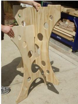
During this process the sides can get hung up so wiggling them back and forth will help the top piece drop down to the bottom.
