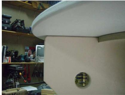
Set the table top on top of its legs. Eyeball the distance of overhang over each of the legs, when it is close enough by the eye, move onto the next step.
