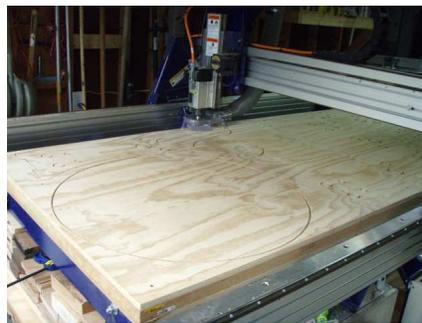
The same applies to the second board during the cutting process. It is always a good idea to keep an eye on the machine while cutting a file for the first time to ensure everything is going as planned.
