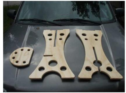
There will be four sets of stools consisting of two sides and a foot rest. Lay them out like the picture above before you are ready to assemble.
