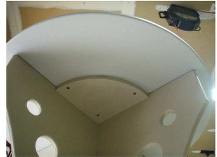
Run three screws into each corner section. Note if you are using 1 1/4” screws and you run them in too deep they can pop up and through the top. Just run them flush with the bottom board.
