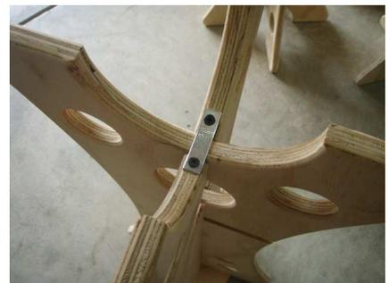
Make sure you install the strapping over the two gaps in the wood. You want to pick up the piece that is flimsy and hold it to the other leg.
