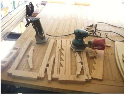
Once the parts have been cut take some time to sand all the edges and faces thoroughly. A routed edge on the outer edges will add some character to the project.
