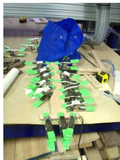
Try to wipe off any excess glue that has squeezed out. Allow glue to setup for at least an hour before removing clamps.
