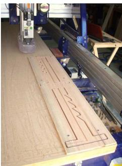
As the file starts cutting the profile of the parts make sure the cut is going all the way through the work piece and into the table surface. If you need to adjust any part of the file make sure you do not remove the hold down or you will loose position.
