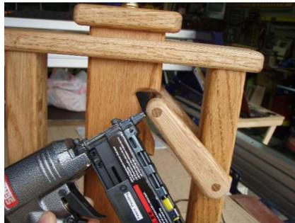
Using a small pin nailer plug a couple pins into the dowels to keep them from falling out. If no pin nailer just dab a little glue in the hole and it will hold just fine.
