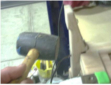
Use the next few pictures to see how the main assembly is glued up. It is the same process as how the ratchet piece was assembled. Above the leg is pushed into place with a rubber mallet.
