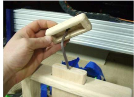
Apply glue to the underside of the top piece and slide it into place.
