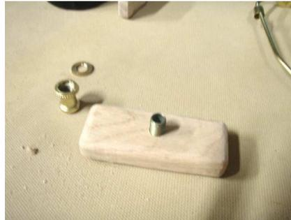
Using a hand drill make the hole just smaller than the diameter of the threaded nipple. This way one can screw the nipple into the wood and use a little epoxy if necessary to hold in place.
