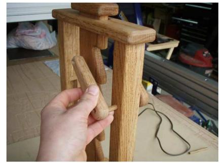
Push the other end onto the dowel and flush that end as well.
