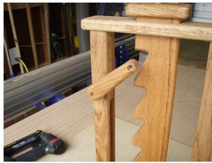
Install one side and flush the the dowel with the lock. Your particular dowel length can be measured by using the thicknesses of your parts.
