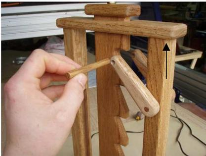
Make sure the ratchet lock is positioned like it is in the picture before inserting the second dowel. Failure to do so will prevent the lock from working properly.
