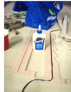
Run the lamp cord through the ratchet pieces. Make sure to spread the glue evenly on both faces. Before applying clamps make sure you look at the next step.
