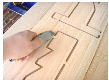
Tab are use to hold all the pieces to the scrap wood attached to them. Use a utility knife to score these edges. Never try to push a piece out without cutting the tab, it will tear the grain on your project. Sand remaining tab flat.
