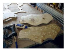
Use a good yellow glue to hold the pieces together. A pin nailer will help keep pieces aligned until the glue has set up.
