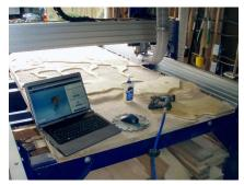
The Autodesk 123D make software labels each slice, so it is nice to keep a computer close by for assembly, this way the user knows which piece connects to each other.
