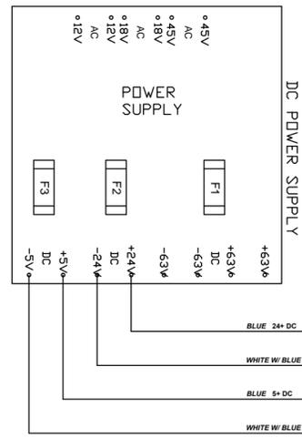
ALL EXTERNAL DEVICES CONNECTED TO CONTROL BOARD TERMINALS ARE PROTECTED BY 5VDC AND 24VDC LOW-VOLTAGE LIMITED ENERGY CIRCUITS
