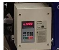
RPM Display of Gantry or Buddy Spindle. When set to Local (Lo/Re) mode, use arrows to change RPM.
