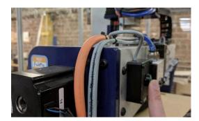
With the green button still depressed, insert a tool holder into the spindle and hold it there. Release the green button. The drawbar will close, capturing the tool holder. Input "7" should light up, and input "8" should turn off.
