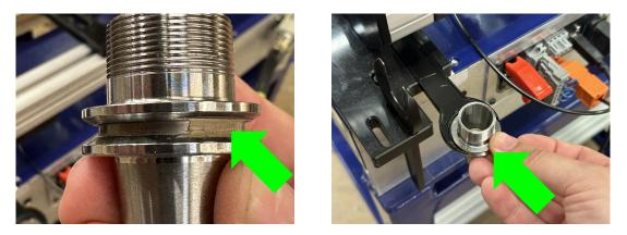
Next, select a collet sized to match the bit that you want to insert into the toolholder. Drop the collet into the toolholder with the longer, tapered end pointing down into the toolholder cone. Place the collet nut on top of the collet and give it a few turns by hand to get it started on the threads of the toolholder.
