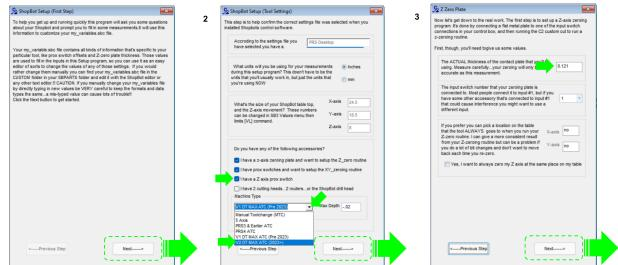
In the "ShopBot Setup (Z Zero Plate)" screen, measure the thickness of the plate and enter that value. Make sure the input switch is set to "1". **DO NOT** check the "Yes, I want to always zero my Z axis at the same place on my table". Click "Next"
