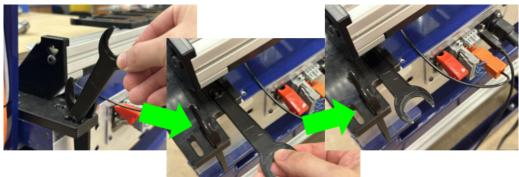
Between the two large bevelled collars on each toolholder, wrench flats have been cut to match the toolholder wrench. Locate these flats and align them when the wrench to slide the toolholder into place with the pull-stud pointing down towards the floor.
