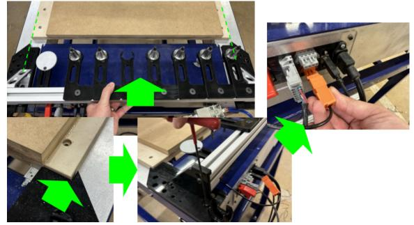
The ShopBot software also give you the option of setting up multiple toolbars that can be swapped on the machine for tools 8-14, 15-21 and 22-28. The installation process for additional toolbars will be the same as the process for installing and removing your main toolbar. Once you've installed an alternative toolbar, you'll just need to run one command in the software to set up for using your alternative toolset.
