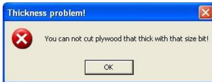
When a button is clicked in the message box , the “value” of that button is saved as a string in a variable named “&msganswer” so that you can use it in an IF test to act on the operator’s answer. The possible values for that variable are...
