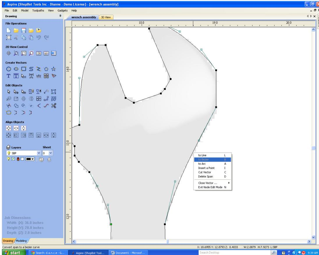
Select both the vectors and component to trim. Switch back to the modeling tab, and select the clear model inside/outside vectors button. To edit the outline vectors, just undo the clearing operation and switch back to the 2D drawing tab. Click on the vector and select the node editing tool to move the vectors towards or away from the edge of the model.
