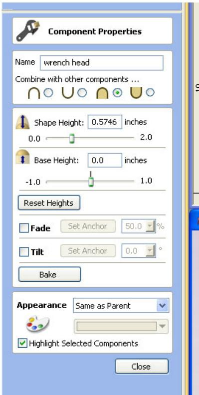
Within the component properties toolbar, it is possible to adjust both shape height and base height. The main difference between the two is that shape height will change the geometry of the component, while changing the base height will simply lift the shape up as if on a platform.
