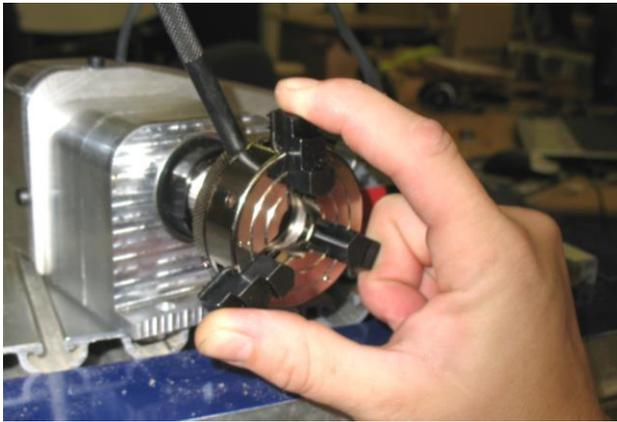
Once you have the jaws in the correct slots, maintain even pressure on each jaw while rotating the knurled ring clockwise. You don't need to apply much pressure, just enough to keep them aligned until the threads catch. Be sure that the jaws are moving evenly towards the center of the chuck. If they seem uneven, reverse direction and remove the jaws to start over.
