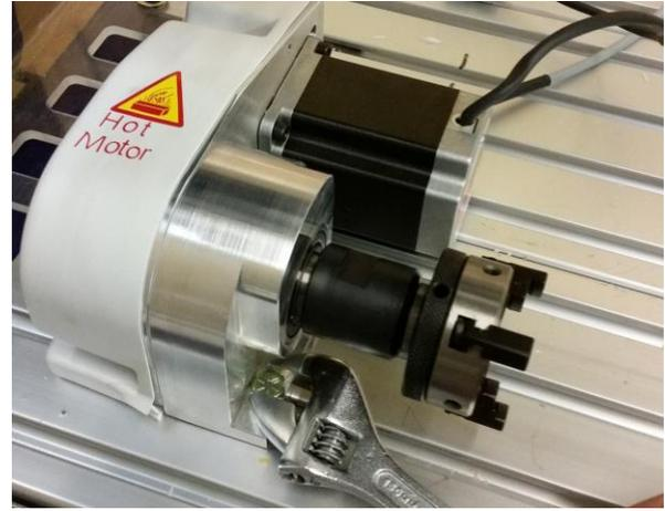
**Tightening the screws on the headstock**
