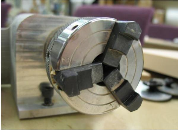
**Chuck jaw configuration: gripping inwards**
