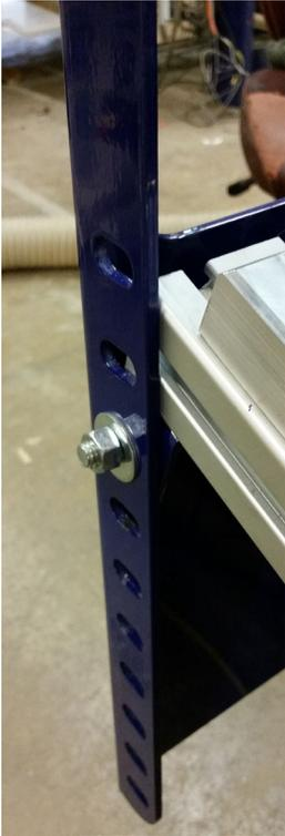
Attach the cross beam using carriage bolts, washers and nuts. For the 6" indexer, the 3rd slot from the top is typically ideal; for the 12", the 7th slot from the top. **DO NOT TIGHTEN BOLTS** - just thread them by hand.
