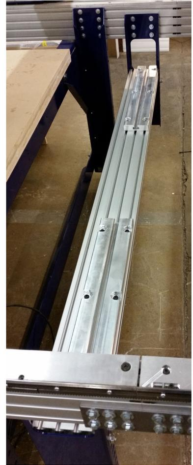
After the carriage bolts are in place, adjust the beam left-right so that it is an equal distance from hanging bracket on either end. There should be about a 1/4" gap.
