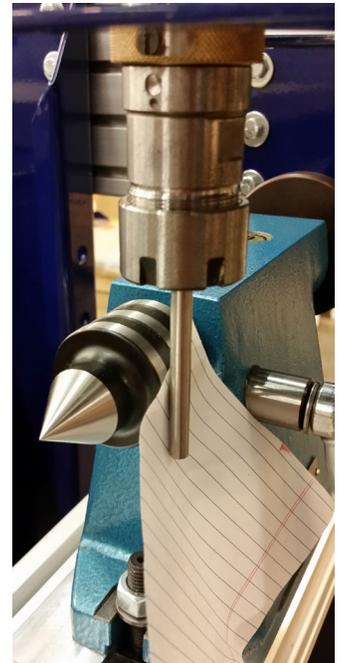
Exit the keypad, and zero the x axis by typing in ZX.
