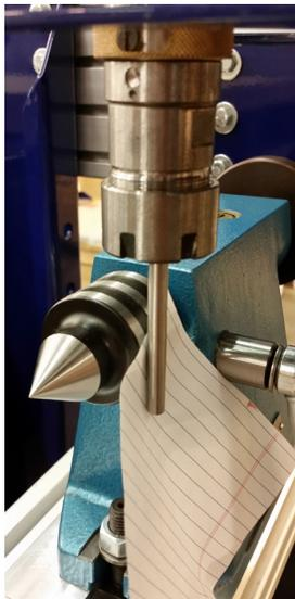
Use the same technique to align the indexer vertically, by bringing the drill rod down from above rather than from the side.
