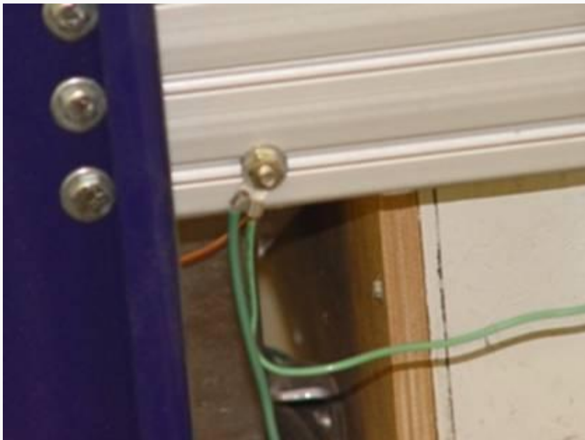
PIC# 4 Short carriage bolt slid into X extrusion with nut and washer
