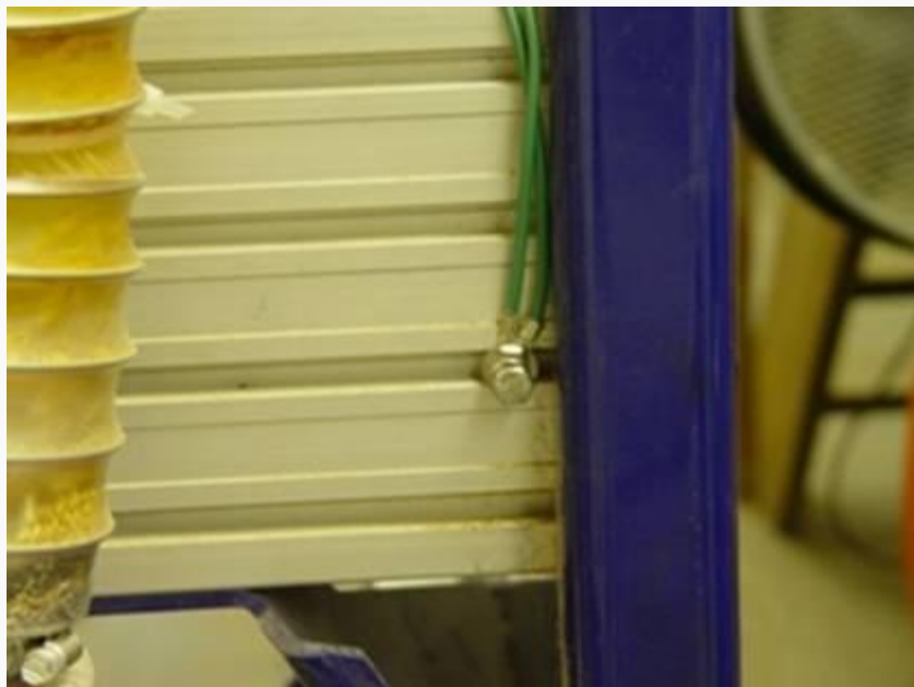
PIC#2 T-nut slid into Y extrusion on the wire entry side attached with short bolt and washer
