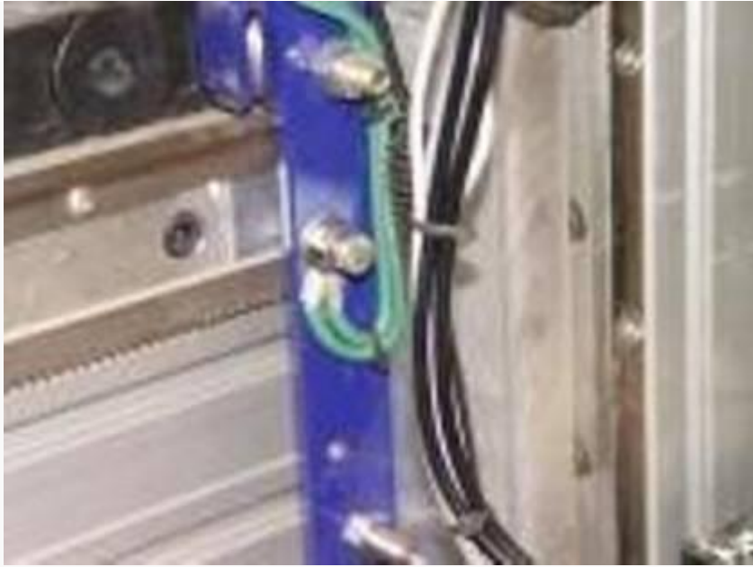
PIC# 3 Attachment at Y car using bolt, nut and washer into tapped hole. Make sure you sand or scrape to bare
