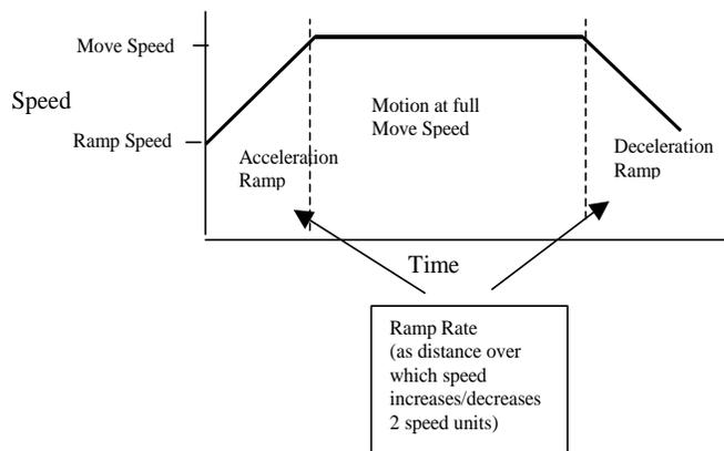
After the start of a move, speed increases during the ramp period from Ramp Speed (the starting speed) to Move Speed for the axis. Motion continues at Move Speed. Then at the end of the move, during the deceleration ramp period, speed decreases from Move Speed to Ramp Speed at which point motion stops. ShopBot's ramps are linear accelerations and decelerations. That makes the overall speed profile of a move a symmetrical trapezoid in time.
