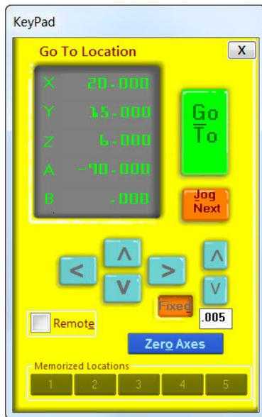
Each axis can be moved using move and jog commands, or the keypad move function.
