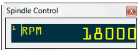
In the main console window, click on “Tools” then “Spindle RPM control.” The Spindle Control window appear.
