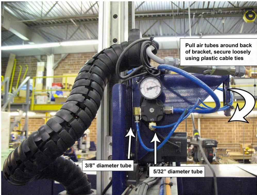
Locate the 1/2" diameter tube that exits the Y axis e-chain on the left side of the machine, and connect it to an air compressor.
