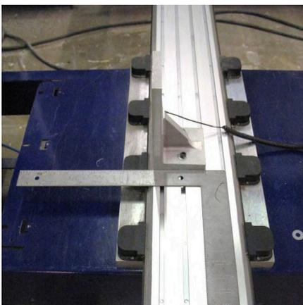
Mount the calibration block onto the PowerStick using a framing square (or similar) to check for alignment.
