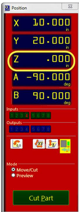
Once the rod is in position on top of the block, exit the keypad and type a **ZZ** command. Check the coordinate window to make sure that this command has been accepted.
