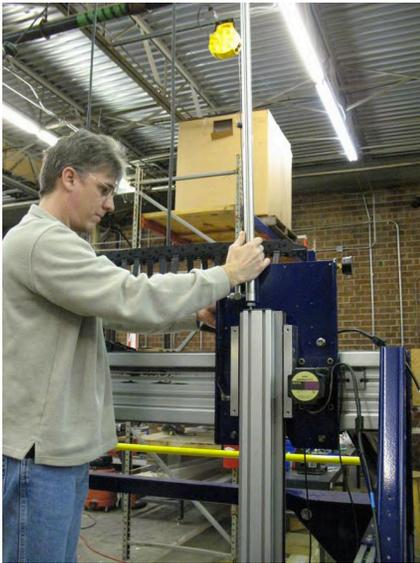
Remove the two 1/4-20 screws from the upper pneumatic assist bracket, and the 5/16-24 screw from the end of the cylinder rod. Mount the cylinder to the front of the YZ car on the left side of the Z-axis extrusion.
