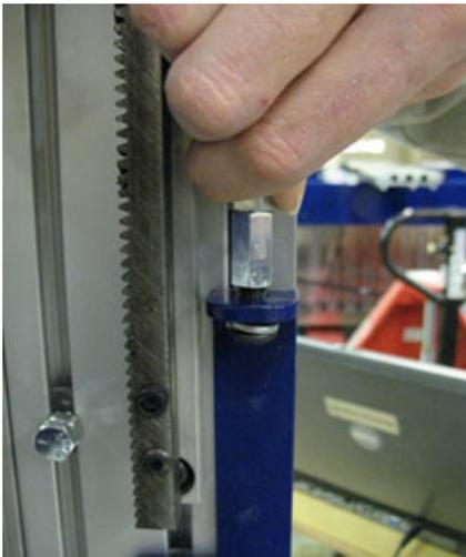
Pull the cylinder rod downward so that it aligns with the tab on the lower pneumatic assist bracket.
