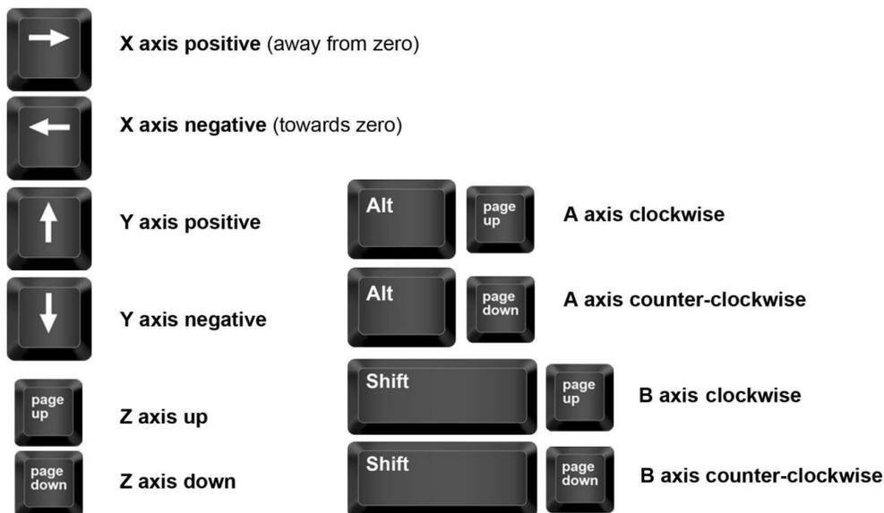
The keypad buttons reflect the actual keyboard. When the keypad is open, the mouse or keyboard can be used to move the tool.
