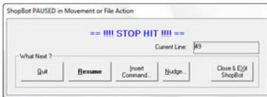
**The best way to stop the machine during a cut is by hitting the space bar on the keyboard.** This will bring the machine to a software controlled stop and following message at left will appear. Choose “Quit” to stop the file and go back to the main console window, or “Resume” to continue the file.
