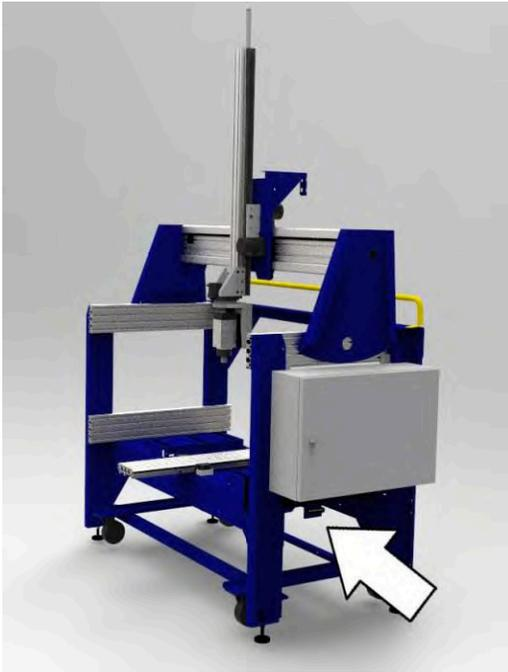
Pull the cam handle (see photo, left) out and to the right. This holds the x-axis motor in the disengaged position.
