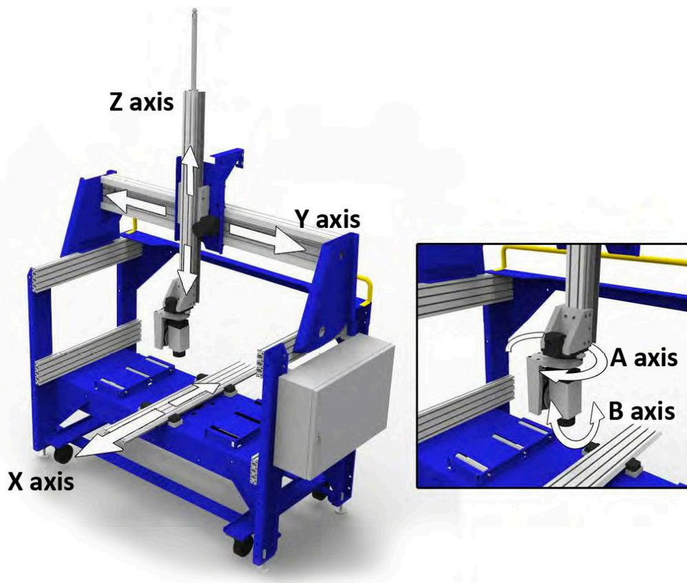
In the image above, notice the position of the spindle. This is referred to as the A/B home position. The spindle is pointing straight down and the front of the spindle is facing the right side of the machine, towards the control box.
