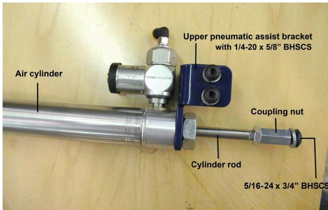
The pneumatic assist serves as a counterbalance for the weight of the Z axis. This reduces strain on the Z axis motor and prevents the spindle from dropping when the machine is powered off.
