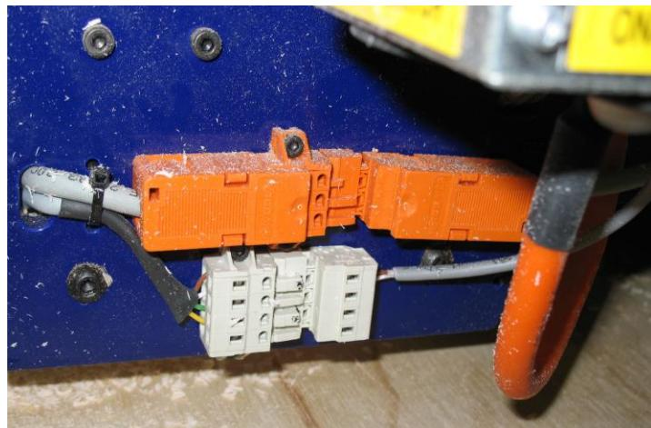
The two loose plugs coming from the bottom of the VFD need to be plugged in at this point. Connect each one to its matching plug on the gantry. Make sure that these connections are tight. Complete the installation by securing the spindle cable to gantry with a couple of zip ties (you may have to cut the old ones out first- just be careful not to cut any of the cables).
