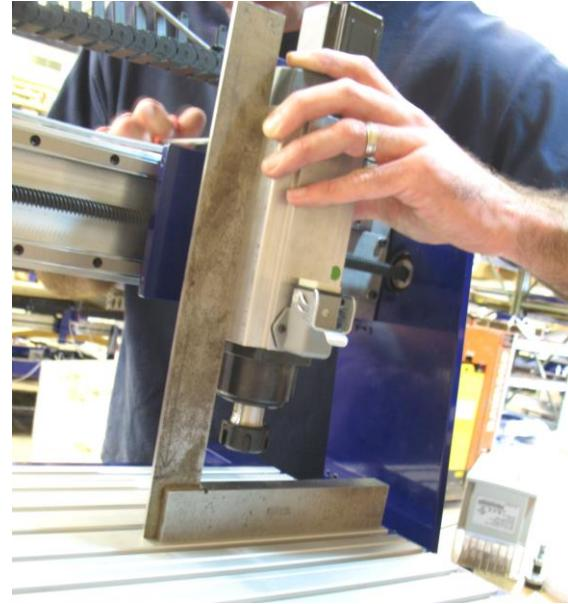
Checking the spindle for square
