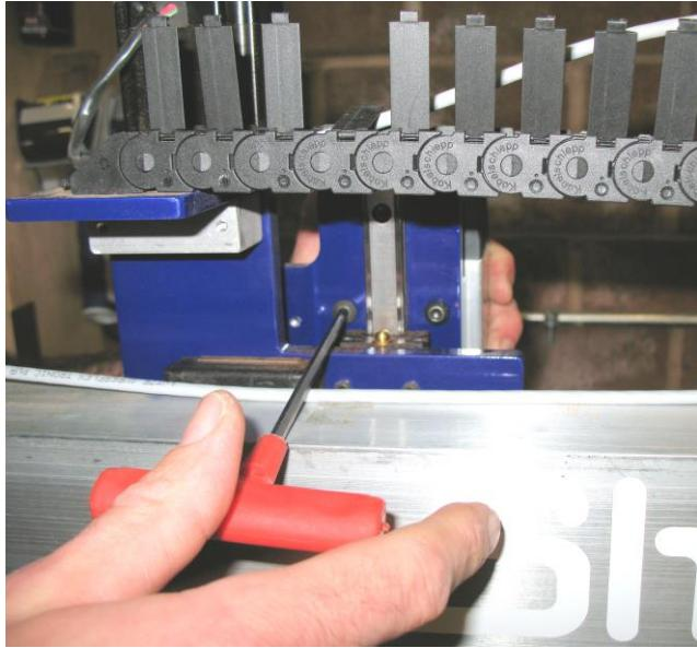
Bolting the spindle to the Z-axis
