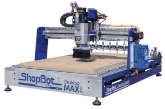
Comes standard with an attached MDF spoil board and is considered our most versatile deck option for a wide variety of machining options. With the ability to fully or partially remove the deck, the open design allows for the use of dovetailing or end-milling attachments.
