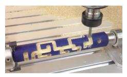
The ShopBot Rotary Indexer allows you to cut full 3-dimensional objects on your ShopBot. Like a lathe, it provides a 4th rotary axis for turning a part, but in addition, provides precise "indexed" control over rotation. With an indexer, not only can you do lathe work but you can also create spindles, newel posts, table legs, 3D sculptures, and more!
