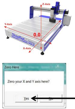
Move the machine to the zero point, and hit "ESC" to exit the keypad mode.
