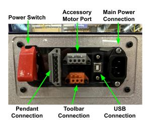
Plug the pendant into the connector on the tool located on the right side of the machine.
