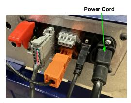
Install power cord into the back of the tool.
