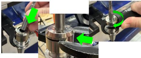
Remove the tool holder from the tool holder wrench. At the toolbar, align the top edge of the tool clip with the same space that the tool holder wrench connects with the tool holder. Gently press the tool holder into the clip with the pull stud pointing upwards.
